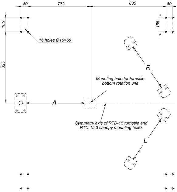
Figure 4. Hole pattern for mounting of the canopy posts (3) relative to the turnstile mounting holes:
