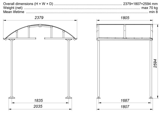
Figure 1. Overall canopy dimensions (frontal view)
