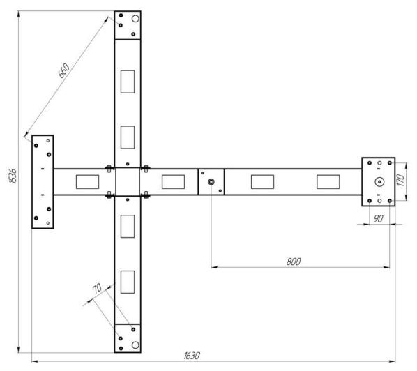
Figure 1. Overall and installation dimensions of the frame
